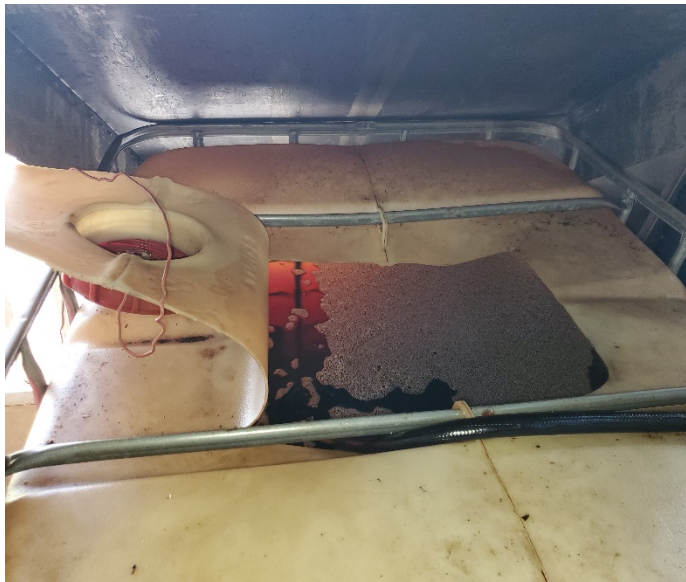
Image showing section of the fuel container cut/removed
